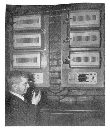
the maximum power output of the inductive transmitters is approximately 35 watts. The receivers of both the space and inductive radio types have an undistorted power output rating of approximately 5 watts. The sensitivity of the VHF receiver is approximately 0.5 microvolts for full saturation of the FM limiter. The sensitivity of the induction radio receiver is approximately 10 microvolts for full saturation of the FM limiter.
